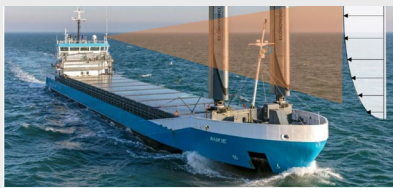
On-board trials & monitoring, including LiDAR wind scan and force measurements
