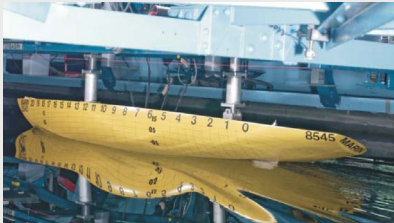
Captive basin tests for hydrodynamic loads with heel, leeway and rudder in the Deep Water Basin
